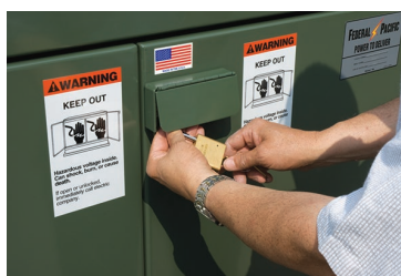
Penta-head (or optional hex-head) actuated door lockbox features stainless-steel hinged padlockable cover to block access to bolt head. Rotate bolt in either direction for opening.
