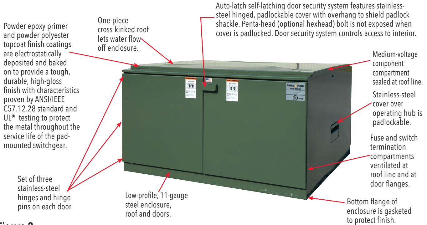
Figure 2 Enclosure integrity and security is assured with Federal Pacific pad-mounted switchgear.
